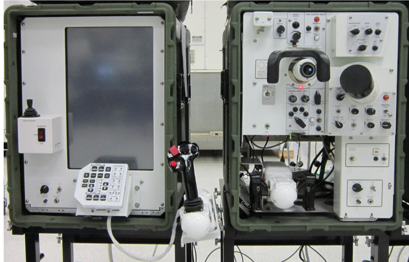
Figure 5: Mounted controls of AGTS
